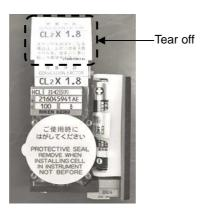
(6) Put the internal case cover and battery unit back in place. For the sensor with a conversion factor label attached, peel off the conversion factor label (product side) removed from the new sensor from release paper and then attach the label in place of the one on the internal case cover.
