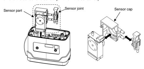
(5) Attach the sensor joint and a new sensor to the sensor cap in reverse order of sensor removal. Insert the connector of the sensor cable to a new sensor and attach the sensor to the main unit. At this time, be careful not to let the sensor cable be caught by the amplifier board. For the sensor with a conversion factor label attached, tear off the product side of the label beforehand.
