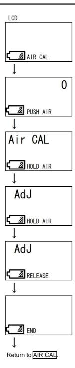
SC-8000 - 14 - 3 Span Adjustment 3-3. Span Adjustment
