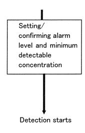
(7) Set up the alarm level and the minimum detectable concentration by pressing MODE switch (below 1 second).
