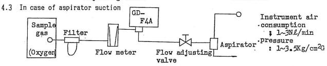
In this method, the reducing pressure degree of detector head must be kept as small as possible and make it at the maximum of -20mmHg.
