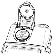
3 Close the detection TAB cover and push the center part firmly with fingers.
