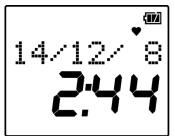
The capacity of the batteries is displayed for about five seconds.
