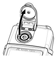
2 Set the detection TAB on the mounting opening.
