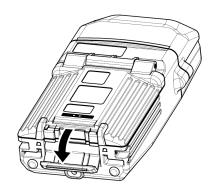
Paying attention to the polarities of the batteries, install new batteries.
