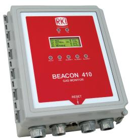
The Beacon 410, four channel, wall mount controller digitally displays the gas name, readings, and status for up to 4 channels. Each channel has 3 fully configurable alarm points. Each channel also has 2 dedicated individual relays for activating external devices like alarm horns, strobes, pumps, fans or other electrical devices. A bank of 5 common relays are also standard. The Beacon 410 powers up to four remote sensors or transmitters.
