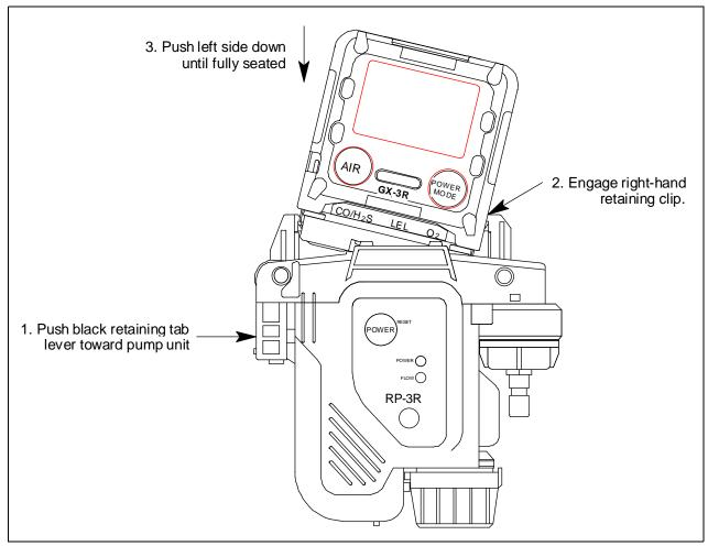
Figure 2: Connecting the RP-3R to the GX-3R
