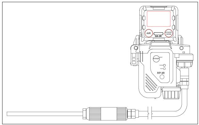
Figure 3: Connecting the Optional Hose and Probe
