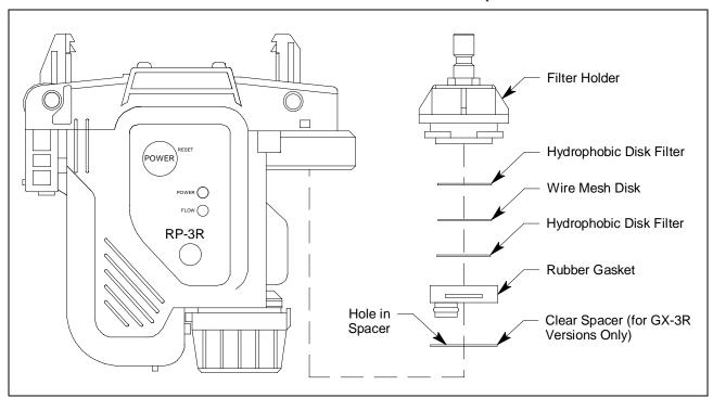
Figure 5: Changing the Hydrophobic & Wire Mesh Filters
