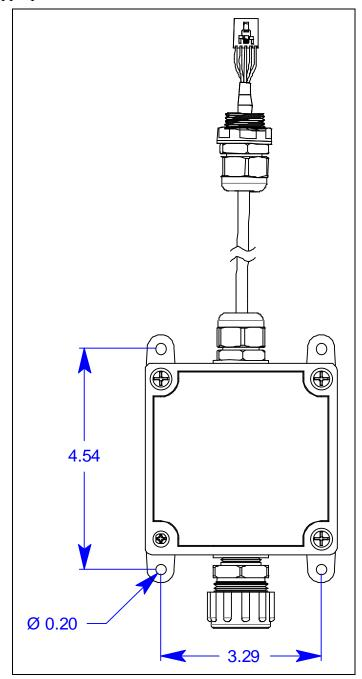
Figure 9: Remote-Mounted Kit's Detector Junction Box Dimensions
