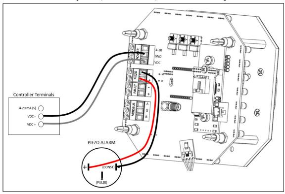
Figure 23: Buzzer Factory Wiring (LED/Buzzer Versions Only)
