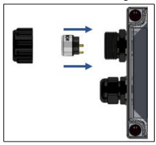
5. Screw the sensor housing cap back onto the sensor housing base, ensuring that the sensor housing cap is only tightened hand tight.
