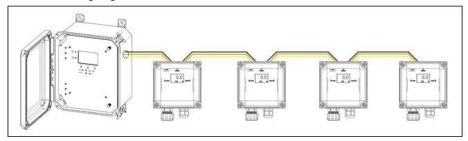
The signal wire of each unit is run to the signal terminal of the neighboring sensor. With each device connected to the previous device via the signal wire, a "chain" is created, with the first device in the chain directly connected to the controller.
