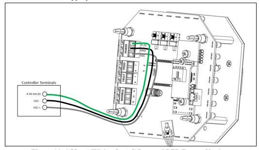
Figure 14: 4-20 mA Wiring for AC-Powered LED/Buzzer Versions
