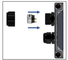
15. Screw the sensor housing cap back onto the sensor housing base, ensuring that the sensor housing cap is only tightened hand tight.
