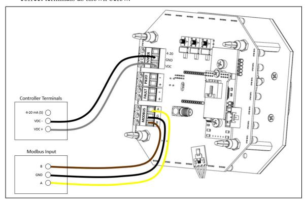
Figure 16: Modbus Wiring, LED/Buzzer Version
