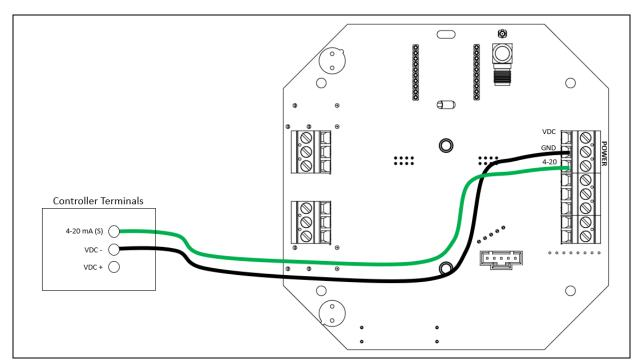
Figure 15: 4-20 mA Wiring for AC-Powered Relay Version
