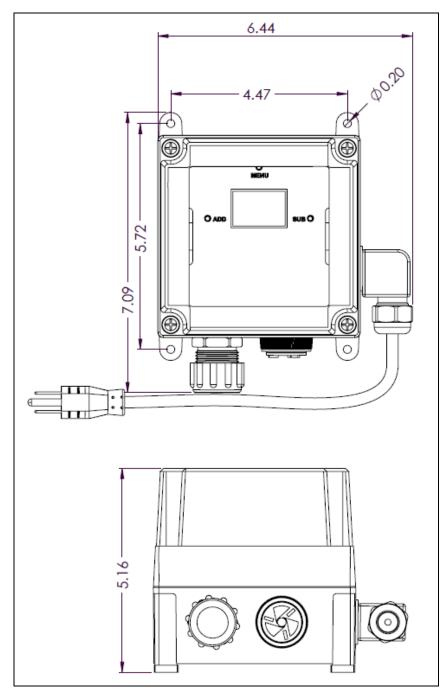
Figure 8: Dimensions for AC Versions with LED/Buzzer Combo
