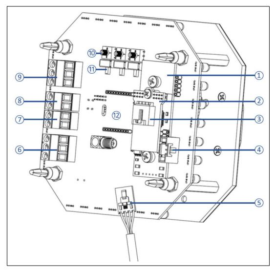
Figure 3: Internal Component Location, LED/Buzzer Version
