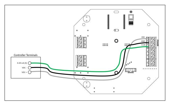
Figure 13: 4-20 mA Wiring for Controller-Powered Relay Version
