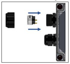
21. Screw the sensor housing cap back onto the sensor housing base, ensuring that the sensor housing cap is only tightened hand tight.
