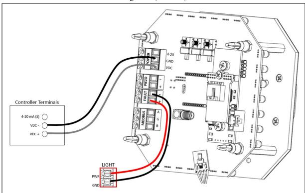
Figure 19: Fault Terminal Wiring, LED/Buzzer Version
