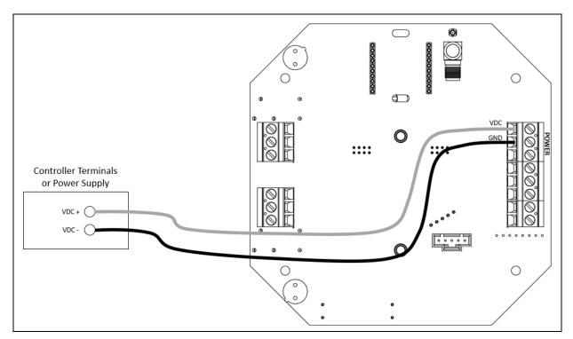
Figure 11: Wiring DC Power, Relay Version
