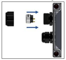
15. Screw the sensor housing cap back onto the sensor housing base, ensuring that the sensor housing cap is only tightened hand tight.
