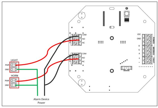
Figure 18: Relay Wiring
