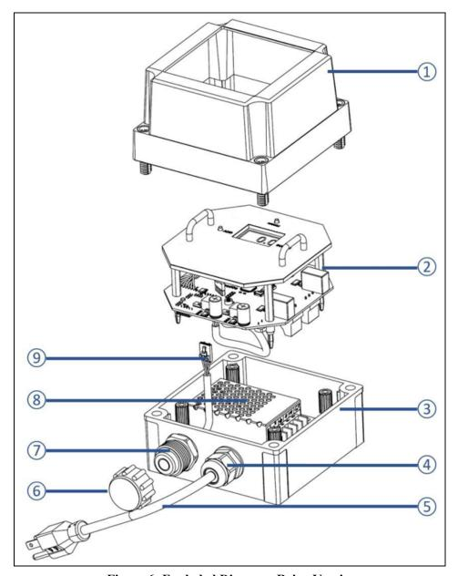
Figure 6: Exploded Diagram, Relay Version
