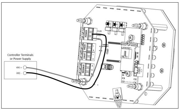
Figure 10: Wiring DC Power, LED/Buzzer Versions
