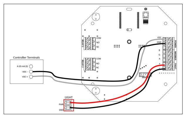
Figure 20: Fault Terminal Wiring, Relay Version
