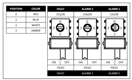
Figure 21: LED and Buzzer Selection Panel
