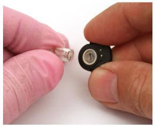
Figure 27: Reinstalling the Electrode Lamp
