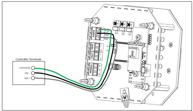
Figure 12: 4-20 mA Wiring for Controller-Powered LED/Buzzer Versions
