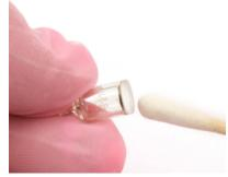
Figure 26: Polishing the Electrode Lamp Window
