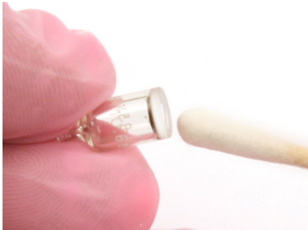
Figure 8: Polishing the Electrode Lamp Window
