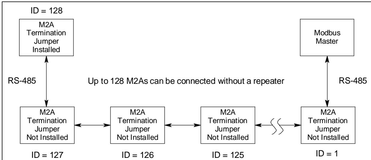
Figure 11: Multiple M2As in a Daisy Chain Configuration
