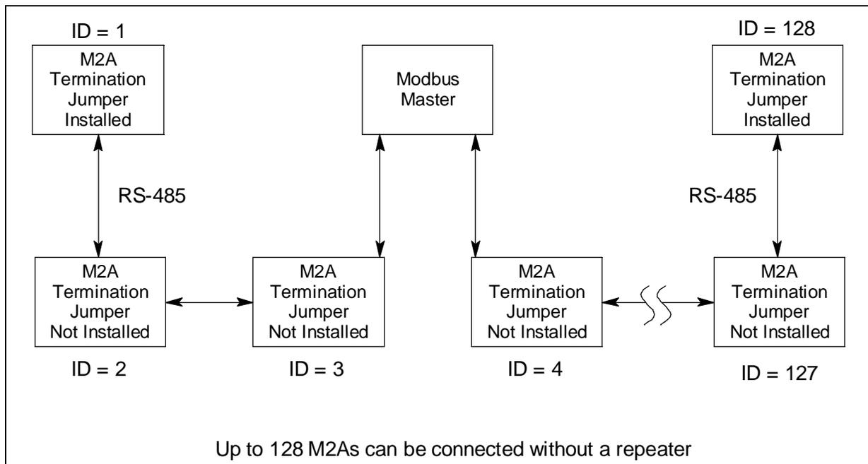
Figure 12: Multiple M2As in a Two Branch Configuration
