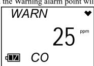
2. Use the AIR button to adjust the Warning setpoint to the desired value.
