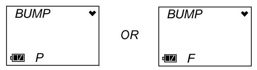
• To view the bump test gas reading, press the AIR button.
