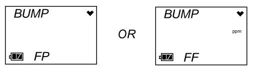
To view the bump test gas readings, press the AIR button.
