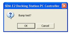
11. The pump will start and the program will indicate that air is flowing. The AIR indicator on the program screen will be on and air will be applied to the instrument(s) for 45 seconds, then the PC Controller Program will perform a zero adjustment on all the channels. The BUMP LED on the SDM-E2 control panel will be flashing amber.
