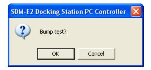
11. The pump in each instrument will start and the program will indicate that air is flowing. The AIR indicator on the program screen will be on. The BUMP LED on the SDM-E2 control panel will be flashing amber. Air will be applied to the EAGLE 2 for 45 seconds, then the PC Controller Program will perform a zero adjustment on all the channels.
