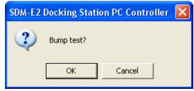
11. The pump will start and the program will indicate that air is flowing. The AIR indicator on the program screen will be on. The BUMP LED on the SDM-E2 control panel will be flashing amber. Air will be applied to the EAGLE 2 for 45 seconds, then the PC Controller Program will perform a zero adjustment on all the channels.
