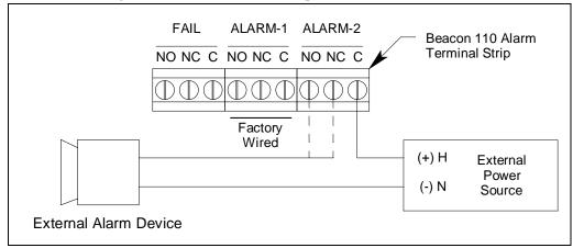
Figure 8: Typical Alarm Device Wiring
