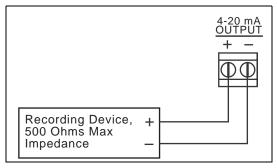
Figure 9: Recorder Output Wiring
