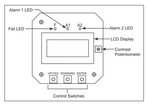
**Figure 4: Control PCB Component Location**
