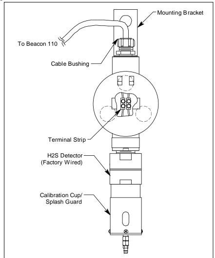
Figure 2: H<sub>2</sub>S Detector Component Location
