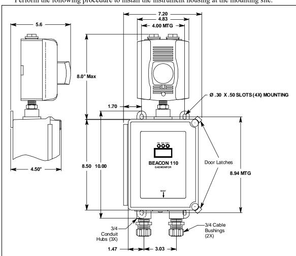
Figure 5: Beacon 110 Rig Monitor Outline & Mounting Dimensions
