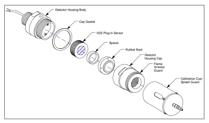
Figure 3: H<sub>2</sub>S Detector Component Location
