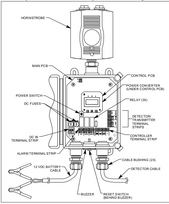
Figure 1: Beacon 110 Rig Monitor Component Location
