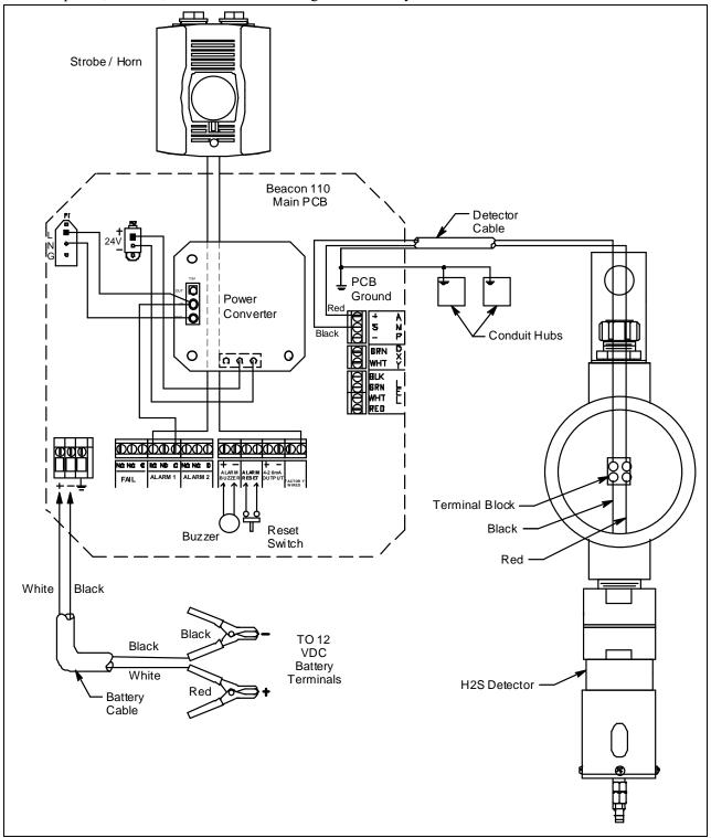
Figure 7: Rig Monitor Factory Wiring
