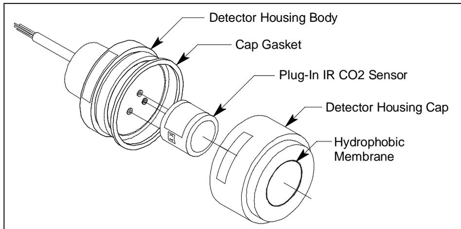
**Figure 2: CO<sub>2</sub> Detector Component Location**
