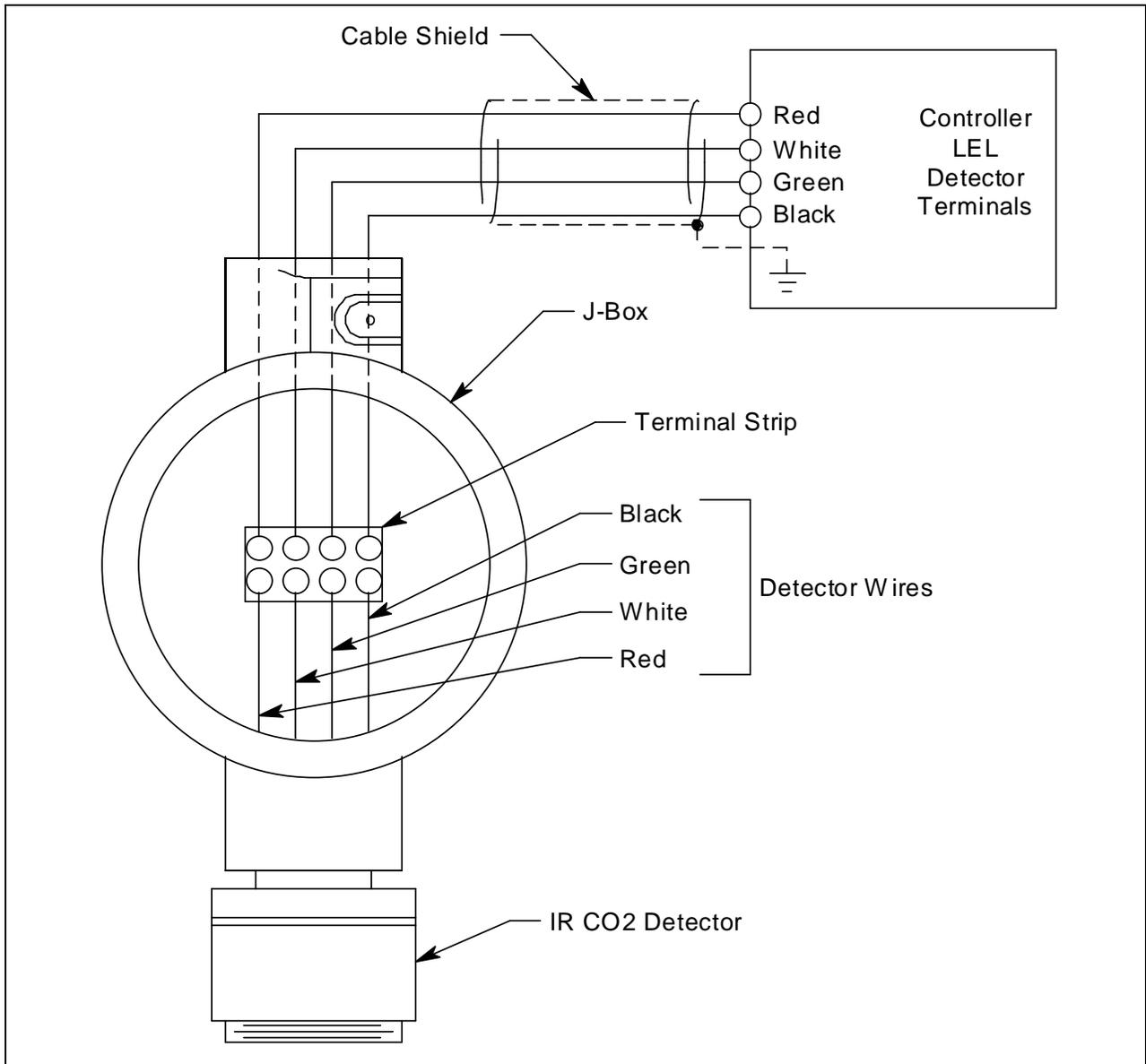
**Figure 4: Wiring the CO<sub>2</sub> Detector to a Controller**
