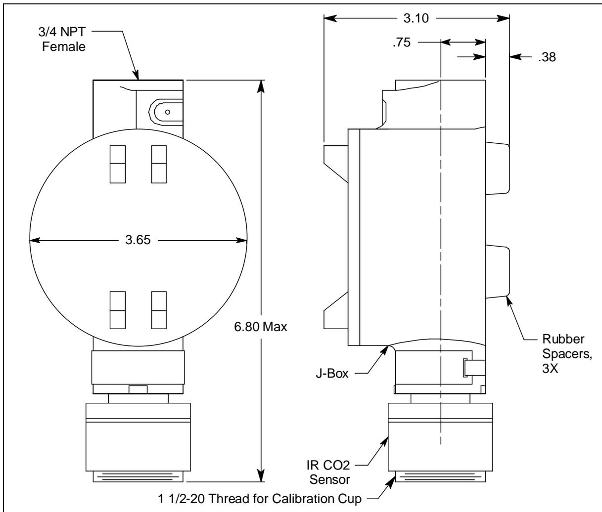
**Figure 3: Mounting the CO<sub>2</sub> Detector**
