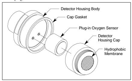
Figure 2: 65-2494RK Oxygen Detector Component Location
