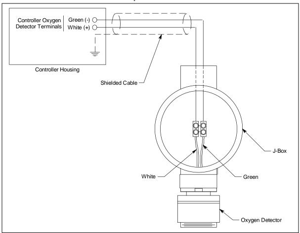
Figure 4: Wiring the Oxygen Detector to a Controller
