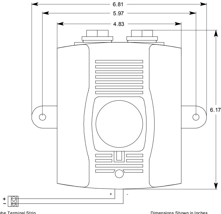
**Figure 6: Horn/Strobe Wiring/Outline and Mounting Dimensions**
