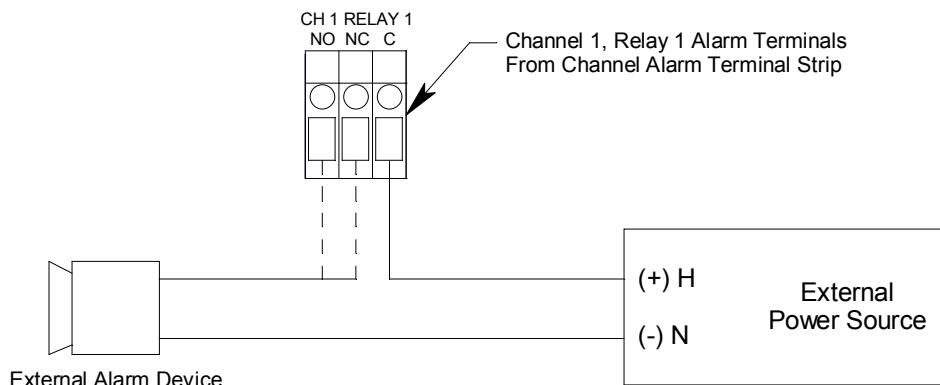
**Figure 11: External Alarm Wiring**
