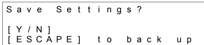
6. To save the global parameter settings, press and release the UP /YES button. The screen will indicate that the Beacon 410 is saving the settings for a few seconds then the Beacon 410 will return to normal operation.
