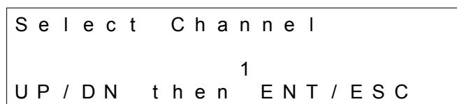
3. Use the UP/YES or DOWN/NO buttons to select the channel whose parameters you want to view and/or update, then press and release the ENTER button. The first channel parameter screen appears and it allows you to select whether the channel is set to **ACTIVE, STANDBY, or, NOT USED**.
