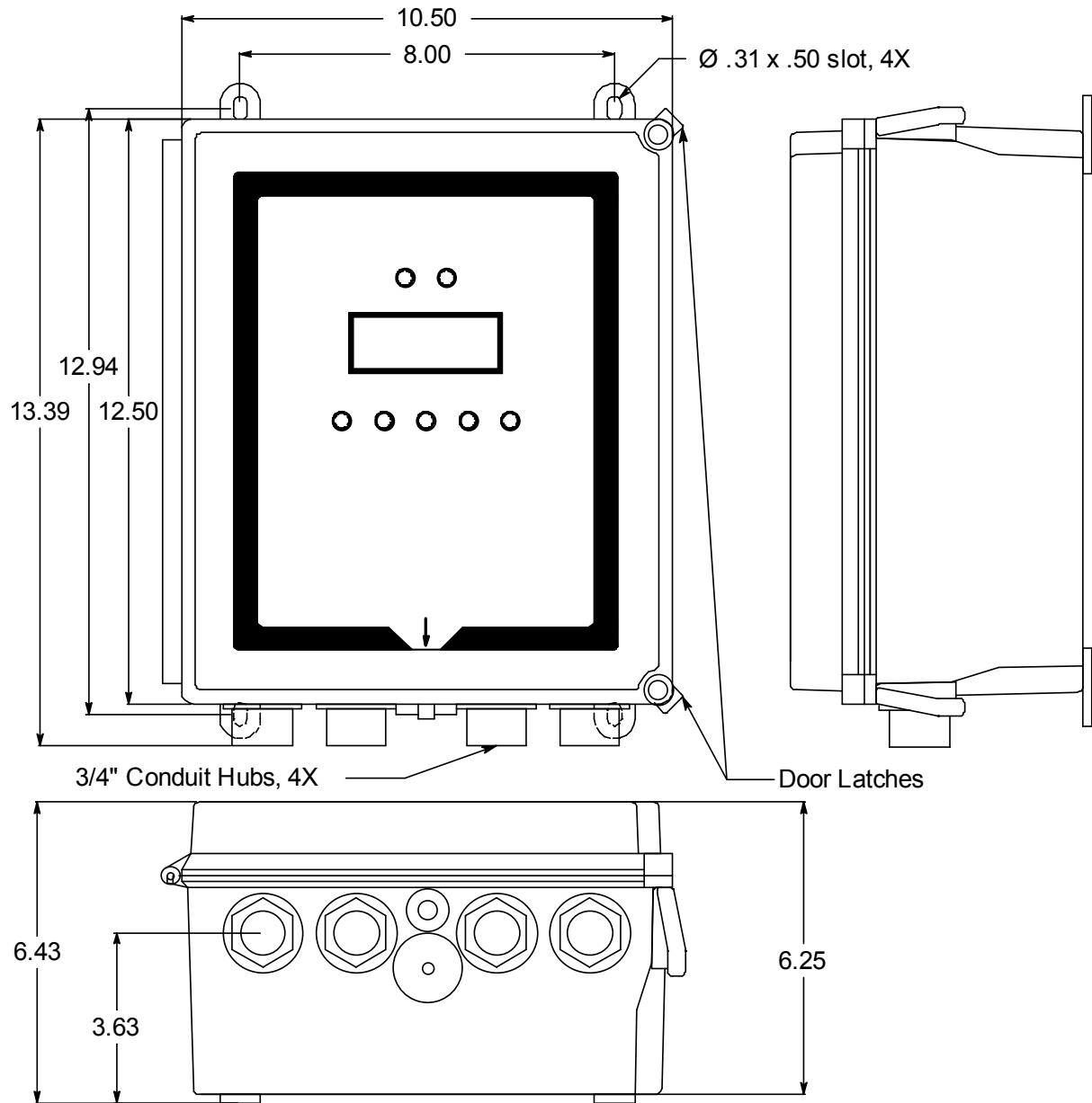
**Figure 7: Beacon 410 Gas Monitor Outline and Mounting Dimensions**
