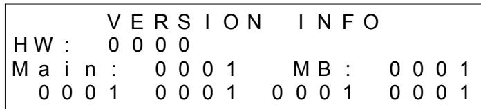
To keep the version information screen on the display longer than a few seconds, press and hold the ENTER button while it is being displayed. When you release the ENTER button, the startup sequence will continue.
