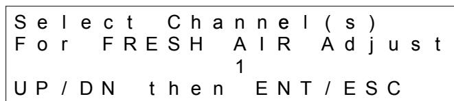
4. Use the UP/YES or DOWN/NO button to scroll through the channel combination choices and select the channel or channels that you will air adjust.
