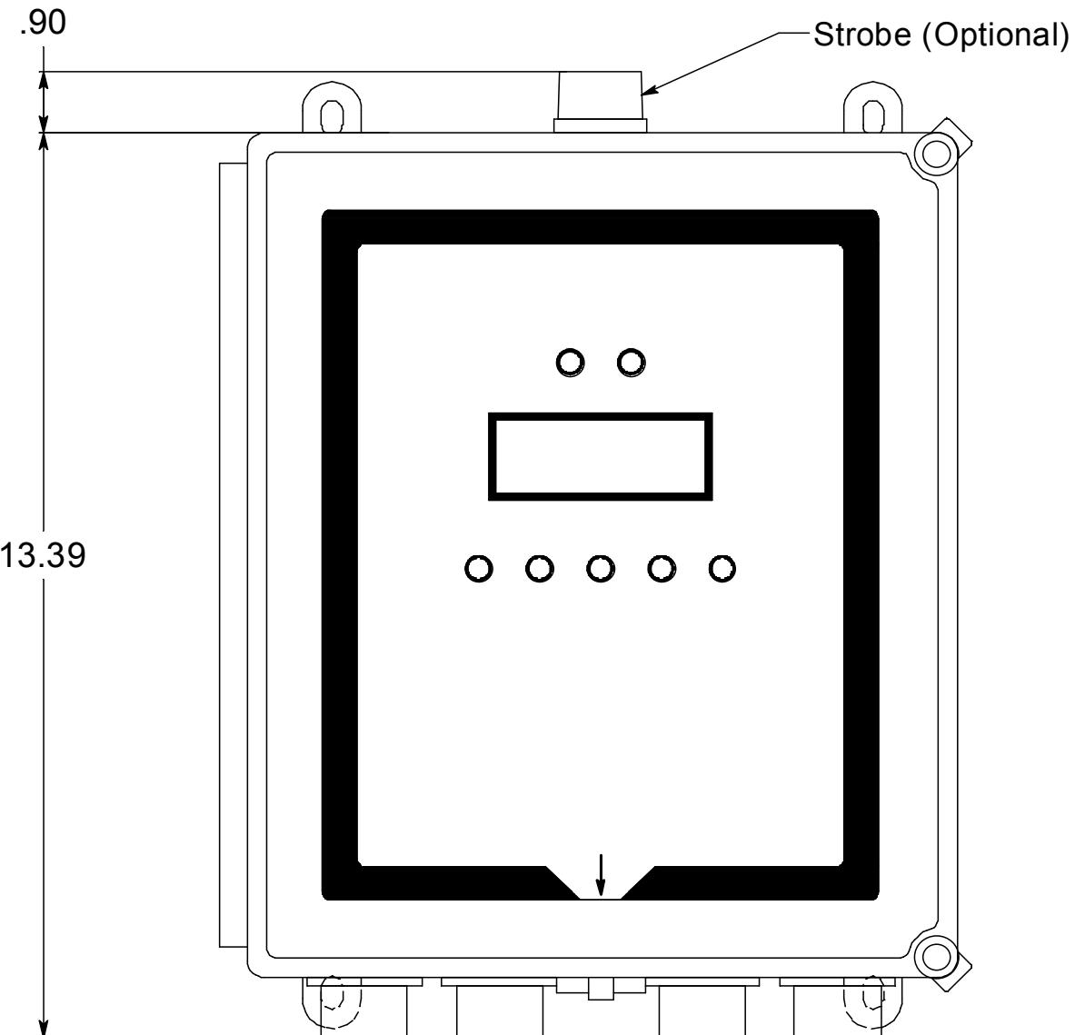
Figure 5: Alarm Strobe Dimensions
