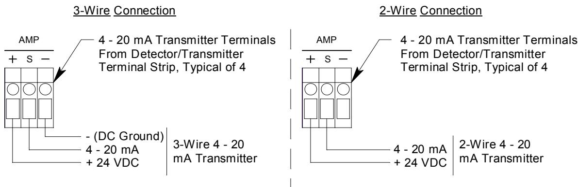
Figure 13: Generic 4 to 20 mA Transmitter Wiring
