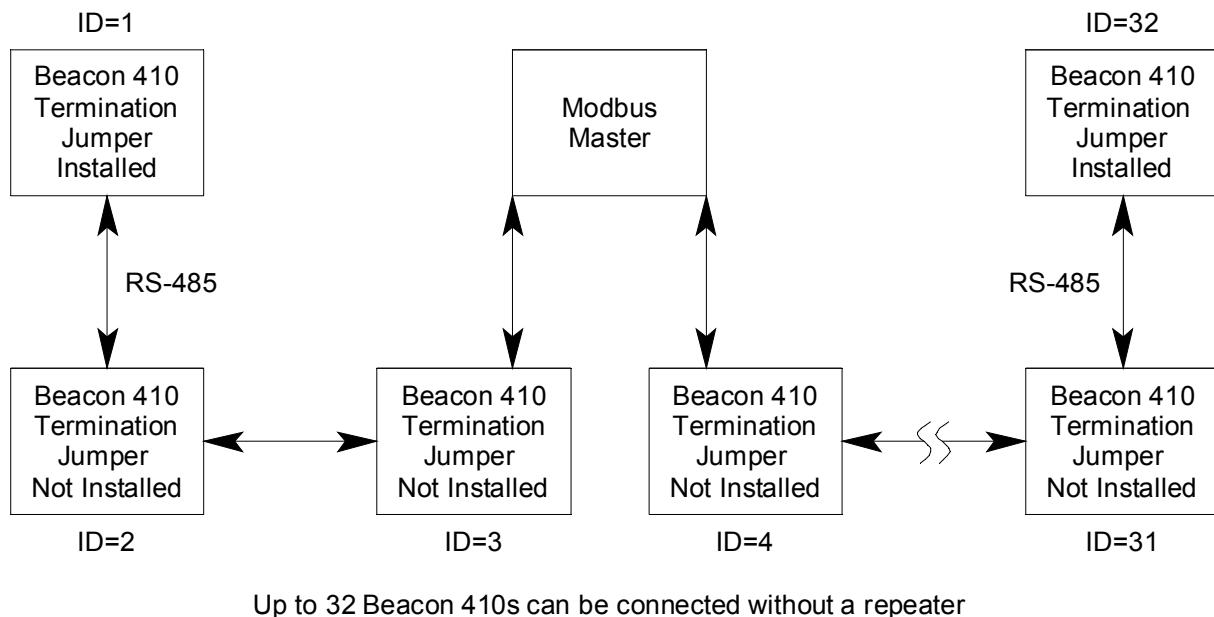
**Figure 16: Multiple Beacon 410s in a Two Branch Configuration**
