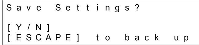
6. To save the channel parameter settings, press and release the UP /YES button. The screen will indicate that the Beacon 410 is saving the settings for a few seconds then the Beacon 410 will return to normal operation.
