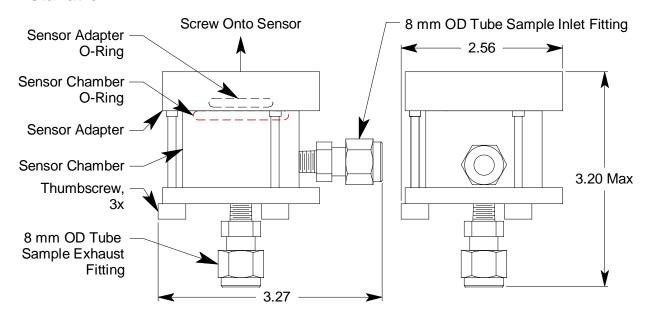
Figure 1: Outline and Mounting Dimensions/Component Location
