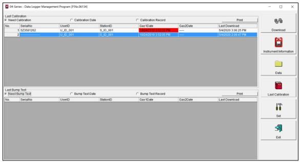
Figure 36: Last Calibration Window: Need Calibration View
