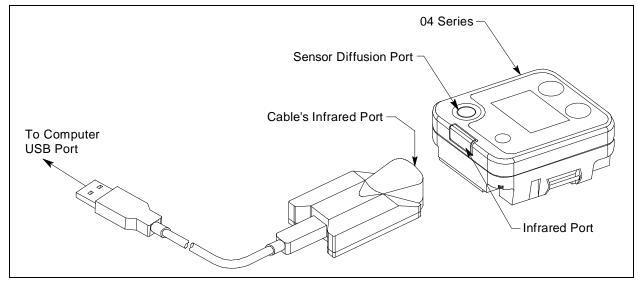
**Figure 6: Aligning IrDA Ports**
