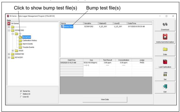
Figure 14: Data Window - Selecting Bump Test Files
