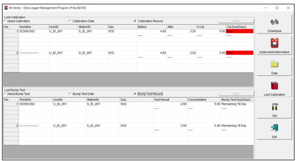
Figure 40: Last Calibration Window: Calibration Record View
