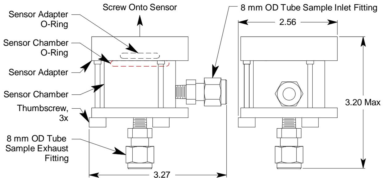
**Figure 1: Outline and Mounting Dimensions/Component Location**
