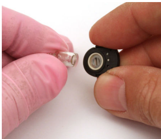
Figure 33: Reinstalling the Electrode Lamp
