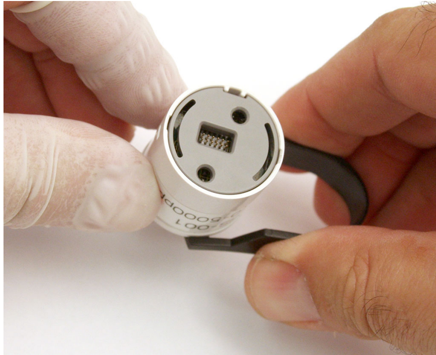
Figure 35: Using Removal Tool
